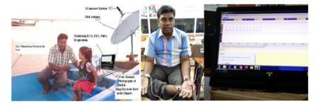
Faculty of RGCET, Mr.S.Saravanan, Department of Computer Science and Engineering, has designed a Telemedicine ambulance Boat with internet communication using antenna system. Biokit is used for monitoring and measuring parameters such as Temperature, Heartbeat, Blood pressure, ECG and pulse signal using computer and mobile through internet.
